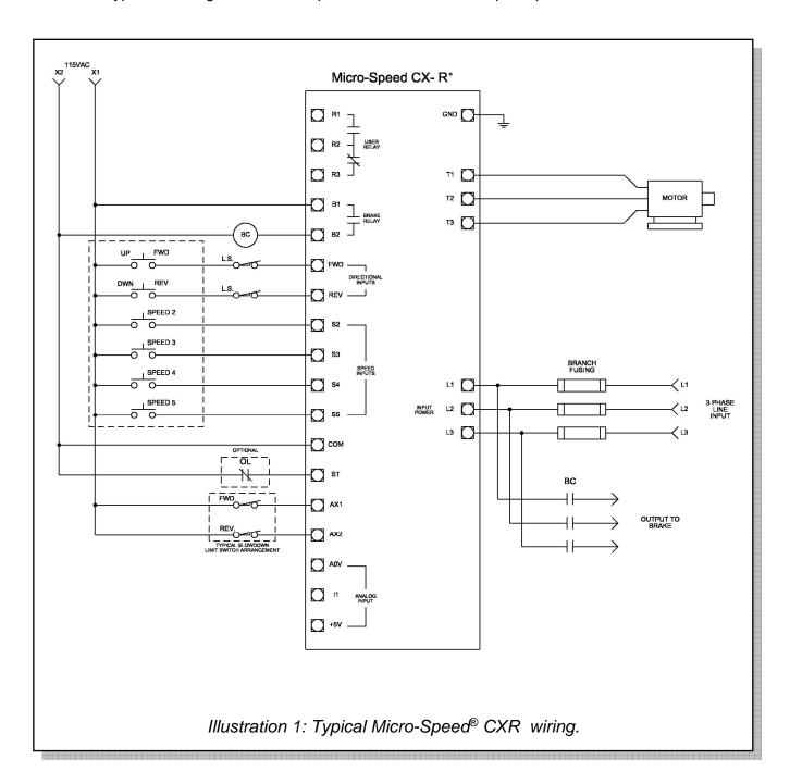
Below is a typical drawing of the Micro-Speed CXRP® with a multi speed pendant.
