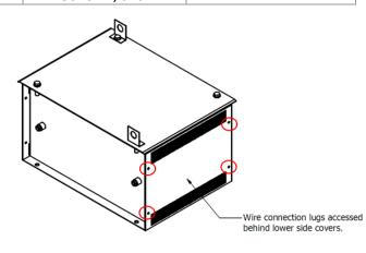
Caution: DO NOT merely run your wires/leads *under* the resistor frame unless you can ensure the wires will not get pinched underneath the frame.
