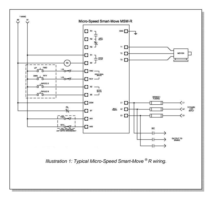
Below is a typical drawing of the Micro-Speed Smart-Move<sup>®</sup> MSM-RP.
