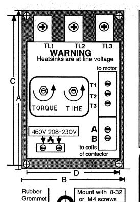
For sizes a,b - Single - piece units (Power Bridge & Logic are in one package). Single-speed is shown.
